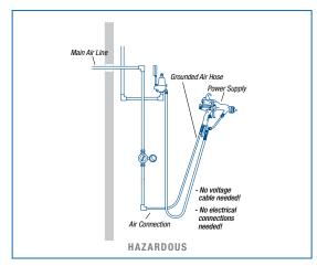
PRO Xs installation is quick and easy requiring very little time. Connect the grounded air hose to the air line and spray!
